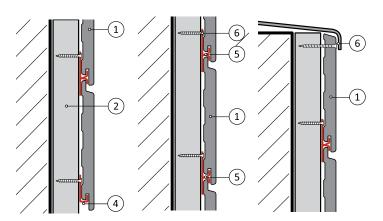
• The connection of the profiles is performed with two base joists side by side or one wider joist and two rows of stan-
